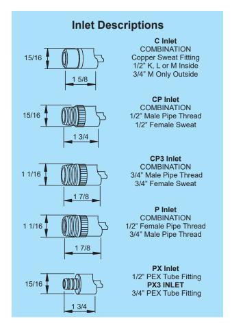
When ordering, specify model, inlet and wall thickness.
