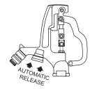
When the hydrant is closed to an OFF position, the diverter will automatically release, allowing the hydrant to drain into the reservoir. The hydrant will drain even if a pressurized or non pressurized hose is attached.
