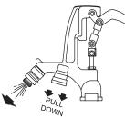
By pulling down on the diverter sleeve during flow, water will be diverted through the backflow preventer (BFP), and allow use with a hose.
