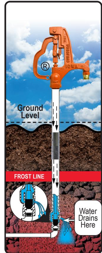
**THE ONLY POSSIBLE CAUSE OF THE BURSTING OF THE HYDRANT HEAD OR TUBE IS AN OBSTRUCTION SUCH AS A HOSE BEING LEFT ON IN FREEZING CONDITIONS OR THE IMPROPER INSTALLATION OF THE PRODUCT THAT PREVENTS THE WATER FROM DRAINING**
