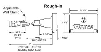
Overall Length = Wall Thickness + Inlet Close Coupled Overall Length = 5"
