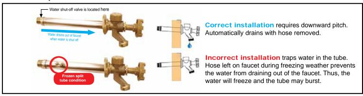
The faucet above is shown with the valve in the closed position. The water is shut off several inches into the home. The water line does not freeze because of the heat in the home. The product cannot freeze because there is no water in the faucet. When the valve is turned off, all of the water in front of the valve drains from the faucet leaving the tube empty. Also shown is correct and incorrect installation and a frozen split tube condition when hose is left on during freezing weather.
