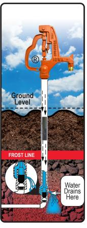
THE ONLY POSSIBLE CAUSE OF THE BURSTING OF THE HYDRANT HEAD OR TUBE IS AN OBSTRUCTION SUCH AS A HOSE BEING LEFT ON IN FREEZING CONDITIONS OR THE IMPROPER INSTALLATION OF THE PRODUCT THAT PREVENTS THE WATER FROM DRAINING
